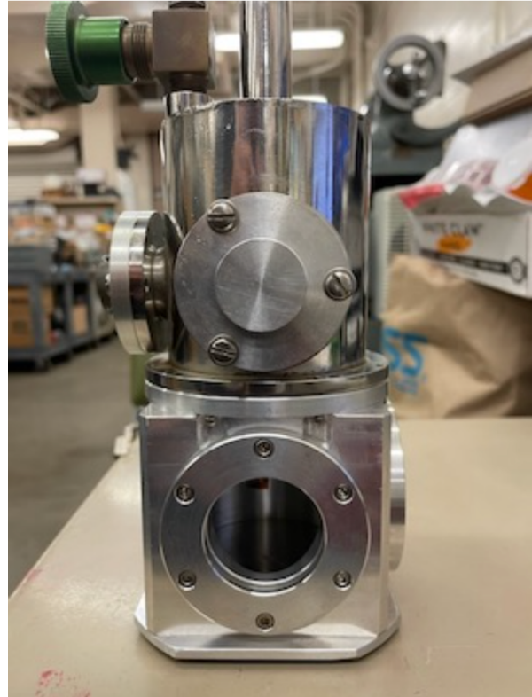
Figure 2 Methane adsorption chamber. Windows are 1.5 inches in diameter for scale.
