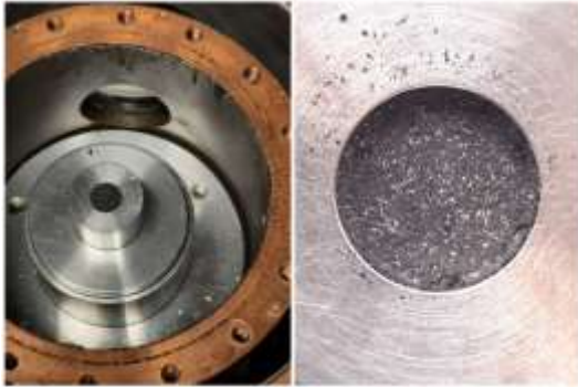
Figure 2. Left: Sample holder with the pressed mixture A3-8 placed in vacuum after heating at 120°C for 2h. Right: Zoomed image of the pressed mixture in the sample holder.
