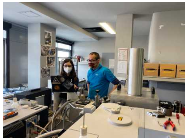
Figure 1. The VEM prototype during measurements at PSL to verify the instrument performance using Venus analogs at Venus surface temperatures.
