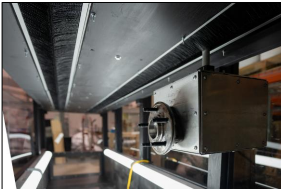
Figure 2. RIDER motor box with wheel hub below the dust mitigation panel and brush system designed to protect the rails above from dust accumulation.
