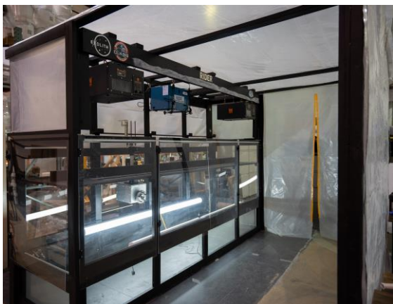
Figure 1. RIDER with motor box, gravity offload system, dust mitigation systems, illumination, and video recording systems.
