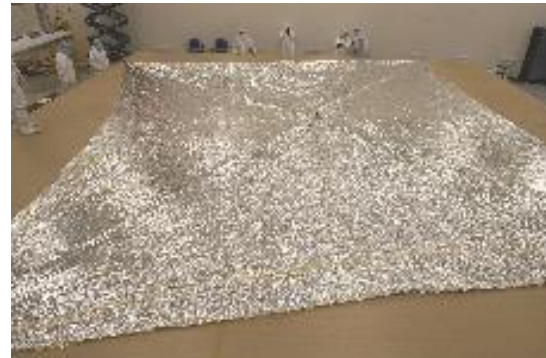
Figure 4. NEA Scout solar sail, unfolded in clean room. Image NASA, Emmett Given.
