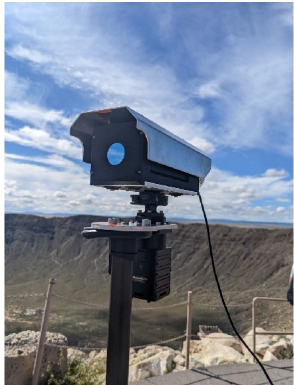
Figure 1: One of two PORIS prototypes, here fielded at Meteor Crater, AZ. The 1 lb. instrument is mounted on a tripod (out of view to the bottom), and includes a compact scan motor controlled by a tablet computer that also collects and processes the hyper-spectral data.
