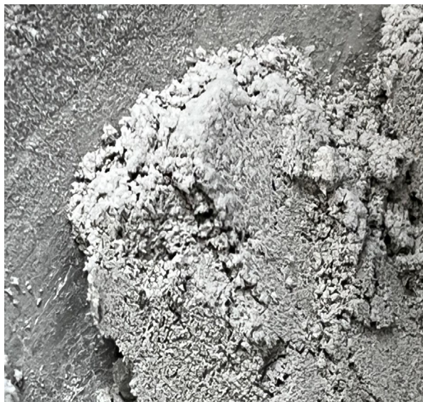
Figure 1. Closeup (field of view \sim 10\text{ cm} by 10\text{ cm} ) view of volatile-bearing cryogenic regolith simulant prepared using NU-LHT-4M. The regolith is combined with LCROSS surface volatile analogs. Adsorbed water crystals (white) can be seen on the outer surfaces of the regolith (grey).
