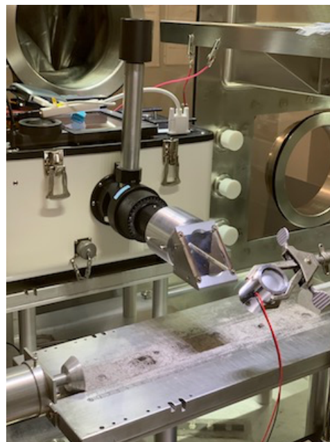
Figure 1. Photograph of the spectral measurement system positioned over the core. Box with clasps is the FTIR. Cylinder with red leads is the IR illuminator.
