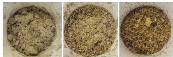
Figure 1: Partially matured SLS developed from plant material and lunar regolith simulant. These represent test samples used to help refine the protocols and provide initial insights.
