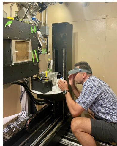
Fig. 1. (upper left) NSI cabinet with computer controller on right. (lower left) Scan setup of large emerald-bearing rock inside NSI cabinet (450-kV X-ray source on left, flat panel detector on right). (right) Dr. Kuldeep Singh (Kent State University) setting up a flow experiment for 4D scanning of calcite dissolution (using the microfocal 225-kV source).
