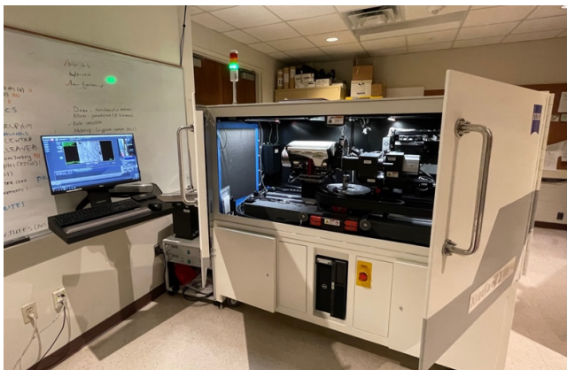
Fig. 3. (left) Zeiss Versa 620 cabinet and computer controller on left. (right) Deben CT5000-TEC in-situ stage mounted inside Zeiss cabinet for leak testing. Source (with filter wheel) on left and detectors on right.
