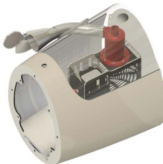
Figure 5: Rendering of the collector integrated in the Kea Atmos payload bay.
