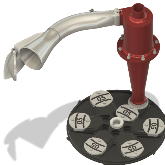
Figure 2: Rendering of intake (silver), cyclonic separator (red) and cartridge (black) with six sample containers (silver circles) for the collector design.
