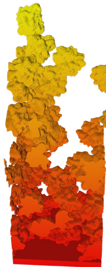
Figure 1: An example for the regolith structure used in the simulations with a porosity of about 0.8 (image from [7]).
