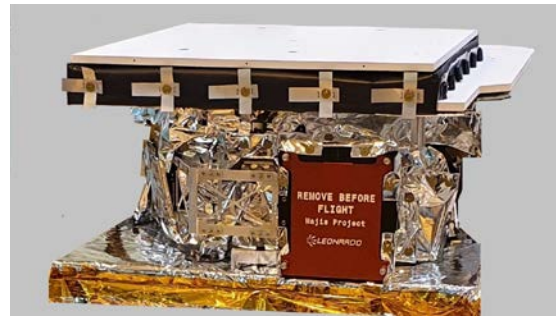
Fig. 1. Optical head of the MAJIS instrument. Dimensions: 912x765x356 mm 3 , 41 kg. The aperture of the optics is protected by a red cover.
