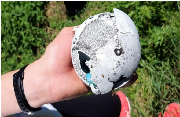
Figure 2. The first 'artificial meteorite' body after the touchdown, thrown from the top of a high building. The inside electronics did not damage, remained reusable. This was our need.
