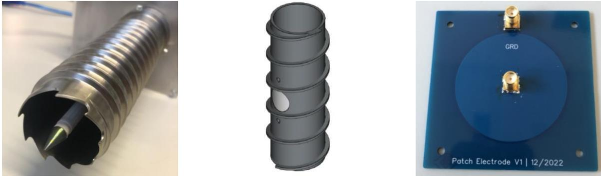
**Figure 1: Pictures and renderings of permittivity electrodes. Left: Lunar Volatiles Scout electrodes: drill shell and heater. Center: PROSPECT permittivity sensor in drill rod. Right: Patch electrode prototype.**
