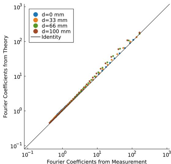
**Figure 2: Correlation between simulations and experiments from insertion depth study.**
