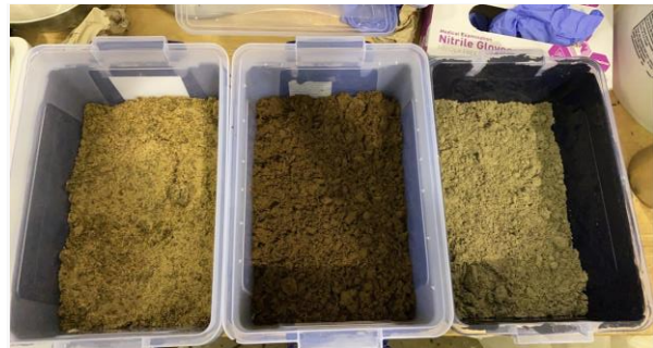
Figure 1: Initial setup of each vermiculture bedding with a 1:1 ratio by volume of desert sand, MGS-1, or LHS-1 (left to right), and composted horse manure.
