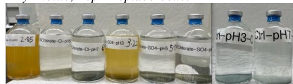
Figure 3: The photographic image of the reactors (Al foil removed) containing smectite and 100 \text{ mmol L}^{-1} chlorate in different \text{MgCl}_2 and \text{MgSO}_4 fluids at pH 3, 5, and 7 (see sample labels) after 30 days of reaction. The last two reactors are control experiments with no chlorate at pH 3 and pH 7.
