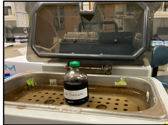
Figure 1: Aqueous solution of Fe (II)/(III), ammonia, and pyruvate, created under anoxic conditions and kept at 70°C in a hot water bath.
