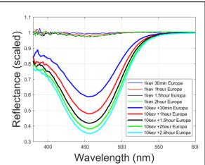
Figure 2. The F-center band and unaffected IR portion of the spectra of hydrohalite when exposed to 1 and 10keV irradiation at 80namps. Thin lines: 1keV. Thick lines: 10 keV.
