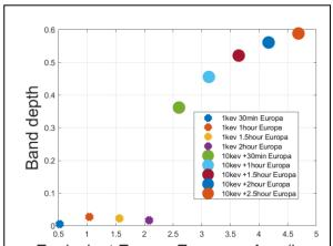
Equivalent Europa Exposure Age (hou Figure 3. The F-center band from 1 keV electrons quickly saturates but doesn't reach saturation for 10 keV electron bombardment, which are more representative of Europa.
