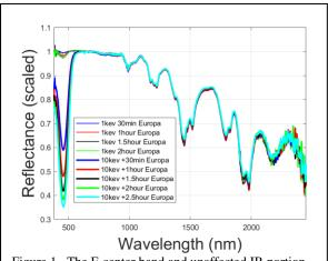
Figure 1. The F-center band and unaffected IR portion of the spectra of hydrohalite when exposed to 1 and 10keV irradiation at 80namps. Thin lines: 1keV. Thick lines: 10 keV.
