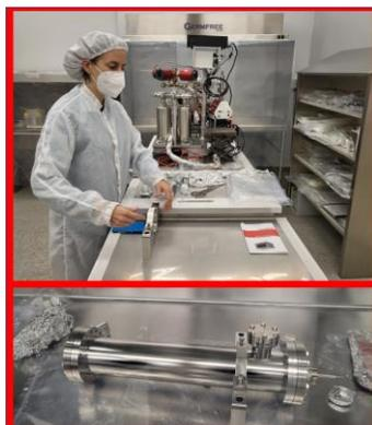
Fig. 1. Manifold (upper image) and piercing tools (lower image) prepared for opening the CSVC in early 2022.
