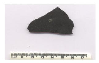
In figure 1 the Aguas Zarcas 3.25 gr slice is shown which we have used for our investigations. A large CAI inclusion can be recognized near the center of the slice.
