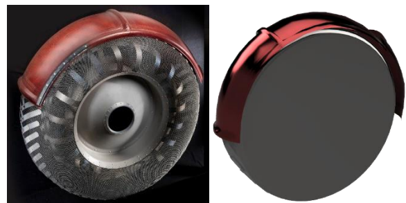
Figure 2 Left- LRV front fender and wheel replicas (credit: Smithsonian https://airandspace.si.edu/collection-objects/wheel-lunar-rover/nasm_A19750830000 ). Right- LRV rear fender and wheel CAD.
