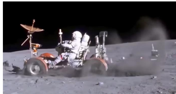
Figure 1 Example rooster tail dust cloud formation during Apollo 16 Grand Prix EVA (credit: NASA).
