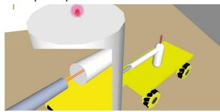
Parts provided by organizers: According to sponsors we want to provide competitors with some parts of the robot: wheel set with four omniwheels, servo motors and batteries.
