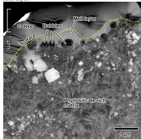
Fig. 2 HAADF-STEM image of a cross section of A0104-02203703. This grain has a melt layer containing abundant bubbles; Most of the tiny bright spots in the melt layer are Fe-Ni sulfide beads.
