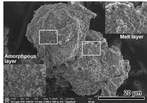
Fig. 1 Secondary electron image of a space-weathered grain C0105-03003800. The upper left part of this grain has an amorphous layer and the lower right part has a melt layer.
