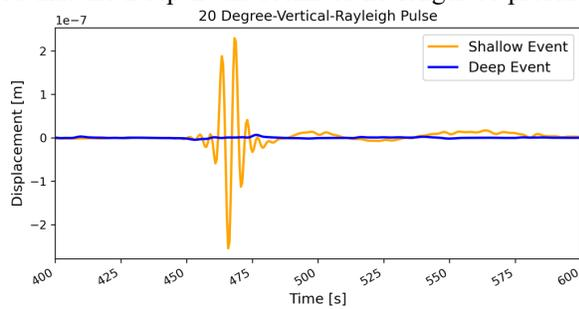
Figure 2. Displacement [m] versus Time [s] for a 20 Degree titanquake, Vertical Component. Both seismograms correspond to events that lack a clathrate lid. The Shallow Event is a 3km quake and the Deep Event is a 525km quake within the rocky interior of Titan. The time interval is from 400 to 600 seconds in order to zoom in on the Rayleigh pulse present within the Vertical component.
