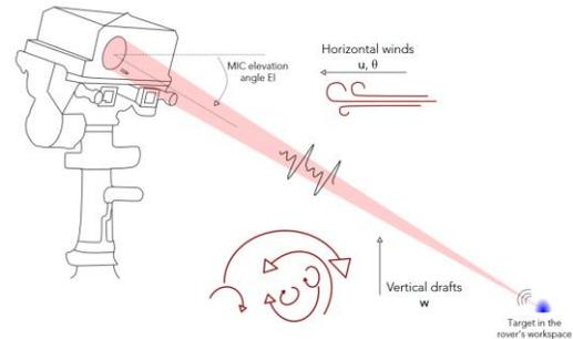
Figure 1 - Sound speed measurement with the SuperCam Microphone
