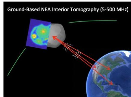
Figure 1: Illustration of ground-based radar tomography.
