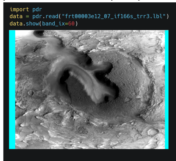
Figure 1. Example workflow for pdr with a CRISM image [2] showcasing the .show convenience method, which allows users to easily view imaging data.
