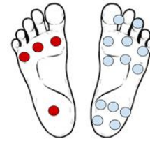
Figure 4: The right shows the placement of the studs on the foot. The left foot indicates the corresponding placements of the piezoelectric ceramic sensors.
