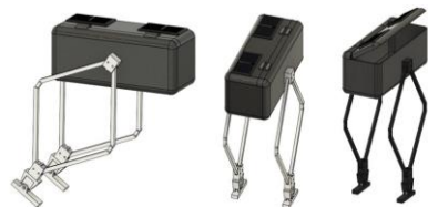
Figure 1: Locust-inspired robot for lunar surface exploration.
