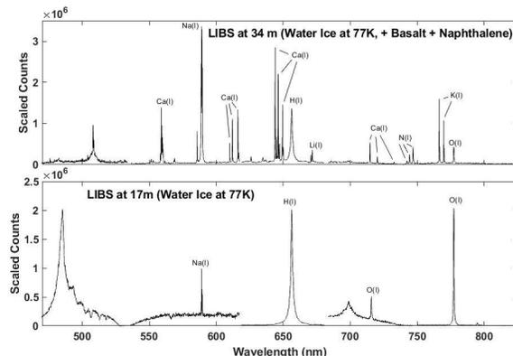
Figure 3: Remote focus LIBS measurements carried out at 17 and 34 m range using a short focal length lens
