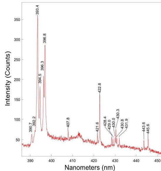
Figure 1: Remote focus LIBS measurement of albite with short focal lens near the sample, 8 meters range, blue spectral range.
