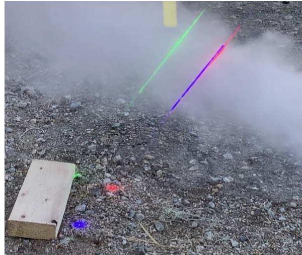
Figure 4. Pre-flight check. Bright backscatter along the beams shown in a cloud of lunar simulant blown in a jet, with beam spots on the ground beneath.
