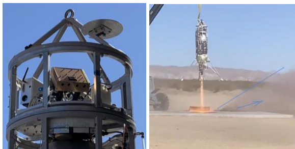
Figure 3. Left: Ejecta STORM on the top of the Xodiac rocket. Right: Flight test blowing simulated lunar soil while Ejecta STORM takes measurements.
