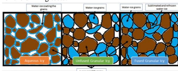
Figure 1: Different forms of cryogenic samples developed for drilling tests.
