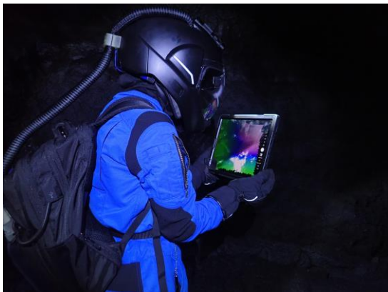
Figure 4: Performing LIDAR measurements in a lava tube while on an analog space mission.
