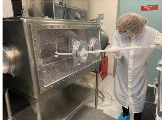
Figure 1. Precision cleaning the glovebox with UPW.
