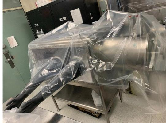
Figure 2. Cleaning procedure completed and the glovebox leak tested using standard gloves.
