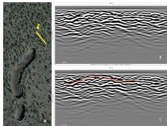
Figure 2: (A) Satellite basemap showing the study area near Giant Ice cave, with one GPR line traced in yellow. (B) 50 MHz GPR data for that line (C) 50 MHz GPR data with interpretations of lava tube ceiling location in red. Interpreted ceiling height is about 3.5 m below the surface with  $v = 0.1$  m/ns.
