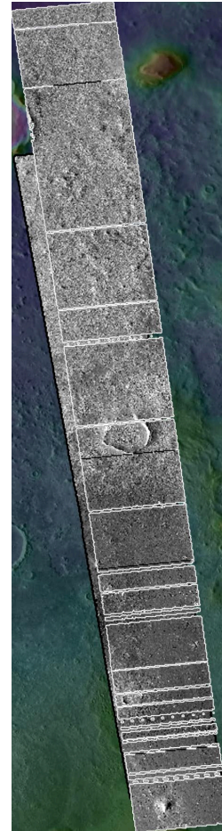
Figure 1. An ERROR orbit (F05_037683_2213) over an OK orbit (B19_017007_2209). We registered individual segments (white outlines) to overlapping data separately, producing distinct translations for segments of the same CTX image.
