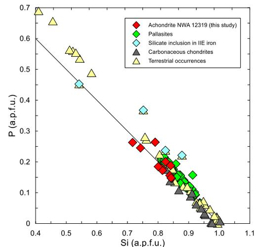
Fig. 5. Linear correlation between Si and P (a.p.f.u.) of P-rich olivine in NWA 12319 and those in the literature [2–12].
