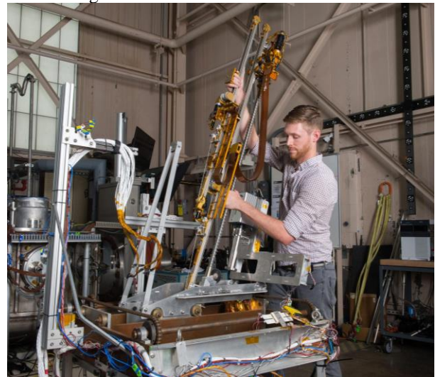
Figure 5. TRIDENTR drill undergoing TVAC tests at NASA GRC.
