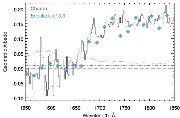
**Figure 3:** The geometric albedo as a function of wavelength for Charon (black line) and Enceladus (blue diamonds; [10]). The dotted line shows the  $1\sigma$  random uncertainty and the dot-dashed line shows the  $1\sigma$  systematic uncertainty in Charon's geometric albedo. When the geometric albedo of Enceladus is reduced by a factor of 3.8 it is very similar to Charon's.
