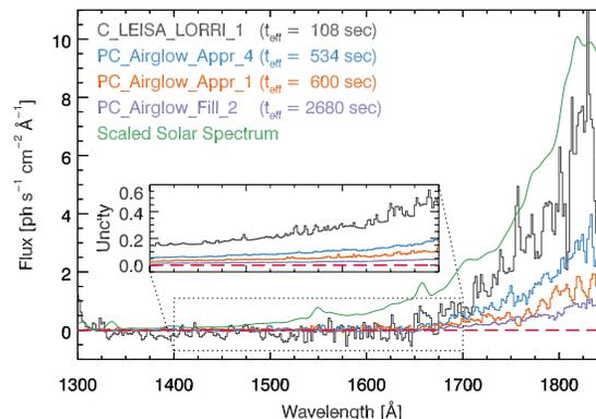
**Figure 1:** FUV spectra of Charon from Alice observing sequences. A scaled solar spectrum is shown for comparison. The inset shows the  $1\sigma$  flux uncertainty for each observing sequence from 1400–1700 Å.
