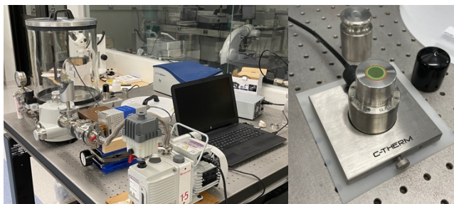
Fig. 1. Laboratory setup at Stony Brook University in the Center for Planetary Exploration Spectroscopy Lab (left). The C-Therm TCi analyzer (right) sits within the bell-jar setup, and butterfly valves hold pressures to within 0.01 mb.
