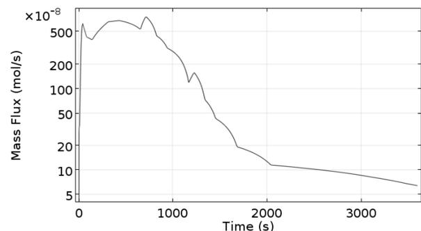
Figure 2: Flux of desorbed water over the regolith's upper boundary inside of the enclosure.
