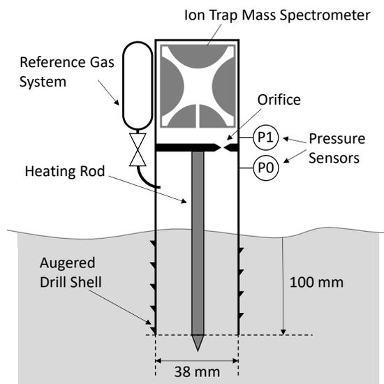
Figure 1: Schematic of the Lunar Volatiles Scout
