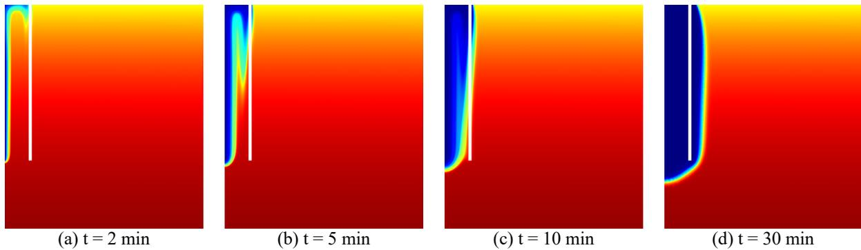
Figure 3: Adsorbed water concentration inside the lunar regolith at different times of the simulation. Blue area represents a concentration of zero.
