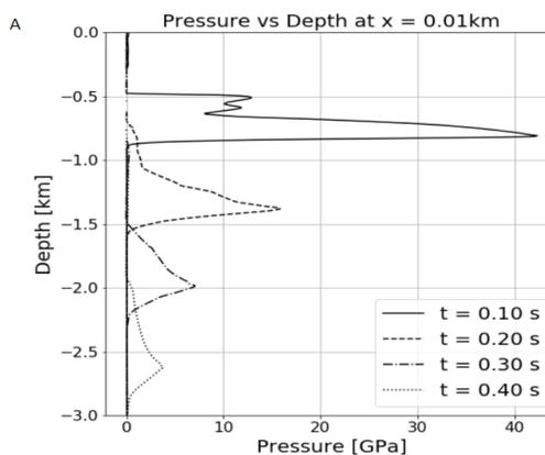
Fig. 5. Evolution of pressure by depth near the center of the crater at 0.1, 0.2, 0.3 and 0.4 seconds.
