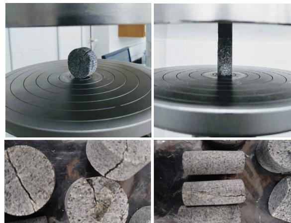
Fig 2. Left: Fractured 1-inch diameter cylinders made from crystalline rim sample after Brazilian test (tensile) was performed. Right: Fractured 0.5-inch diameter cylinders after compressive test.
