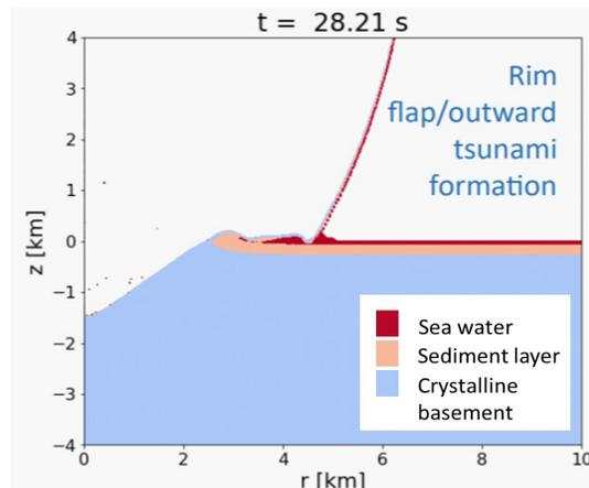
Fig. 3. Density profile at 28.21 seconds as predicted by iSALE, showing rim flap formation and consequent formation of outward moving tsunami waves.
