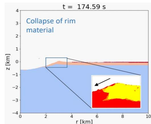
Fig 4. Density profile at 174.59 seconds, showing sedimentary material from rims moving back into the crater. Inset figure shows the direction of the velocity in the x direction. Red and yellow represent the horizontal component of the velocity in the negative and positive X-direction respectively.
