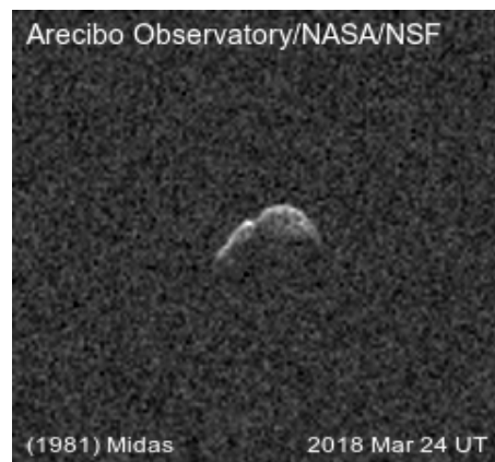
Figure 2: Delay-Doppler image of NEA 1981 Midas observed on 2018 March 24. The Doppler frequency is plotted on the horizontal axis and the delay is on the vertical axis with resolution of 0.954 Hz and 0.5 \mu s (75 m), respectively.
