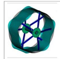
**Figure 3 We use a meshed wheel finite element model: diameter = 250 mm ; width = 100 mm. Thickness of the grouser = 2.5mm; diameter of the central shaft= 5 mm. Parts of the wheel are modeled using aluminum (Young's modulus=69 GPa, density = 2700 kg/m<sup>3</sup>, Poisson's ratio = 0.33). The spoke has a cross-section =10x10 mm<sup>2</sup>. Simply supported boundary conditions are applied at the two ends of the central shaft with no external loading.**
