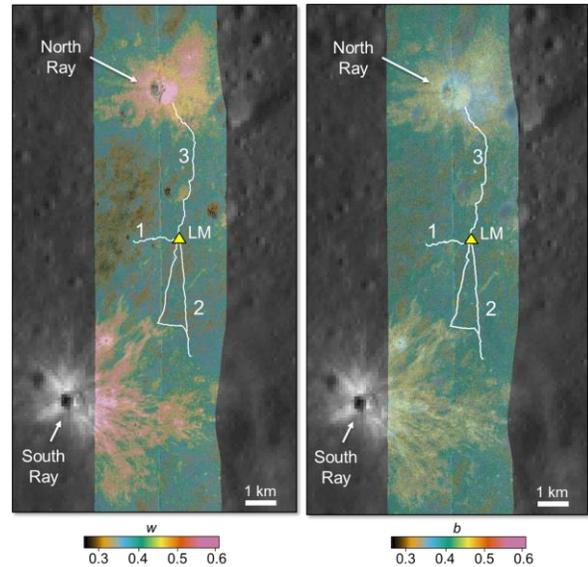
**Fig. 1:** LROC NAC-derived  $w$  (left) and  $b$  (right) maps of the Apollo 16 landing area, showing variations in local geology and regolith properties. White lines indicate EVAs, yellow triangle represents the Lunar Module.
