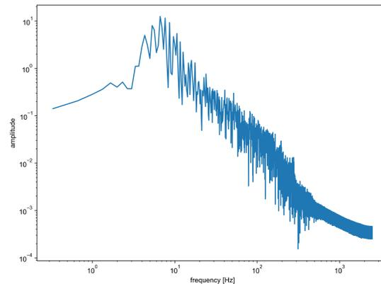
Figure 2: Vertical frequency spectrum for a 60-m impactor striking a 1-km wide asteroid at 100 m/s, recorded 2 m under the surface at the equator of the asteroid.
