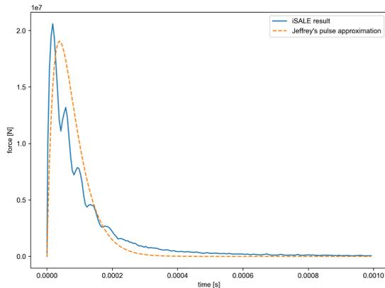
Figure 1: Source-time function calculated for a simulation of 1-kg impactor striking the Martian surface at 1.93 km/s (blue solid line) and a best fit Jeffrey's pulse (dashed line).
