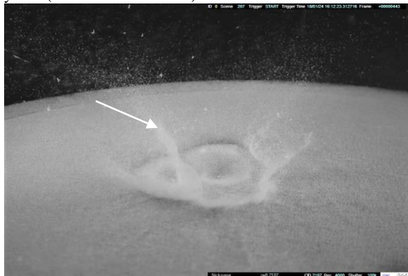
Fig. 3. A frame from an EPIC impact experiment at the INTA-CSIC. A white arrow indicates a ray formed by collision of two impact ejecta curtains.
