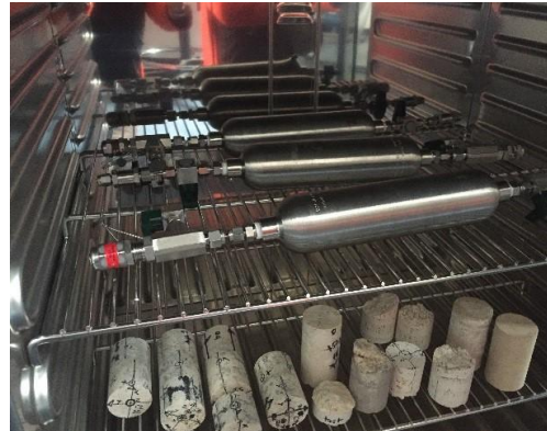
Fig. 1. Batch reaction vessels capable of 15 MPa pressure and up to 80 °C for a wide variety of rock and fluid types, as well as fluid sampling for further analysis.
