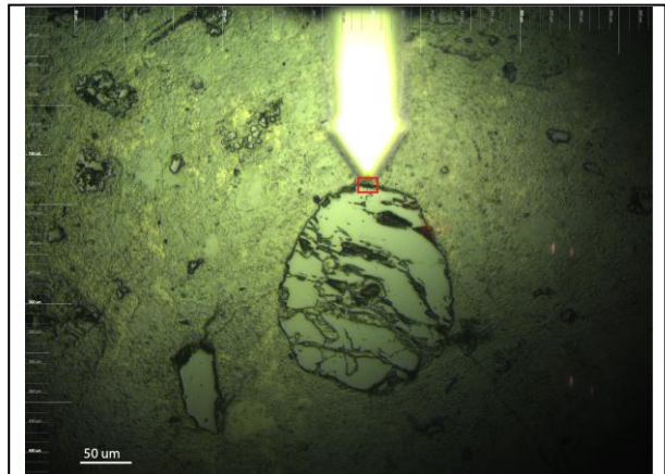
Figure 1. Reflected light image of ALH 83100; Tip of gold arrow shows AFM cantilever position; Red box shows chondrule-matrix boundary where nano-IR measurements were made.
